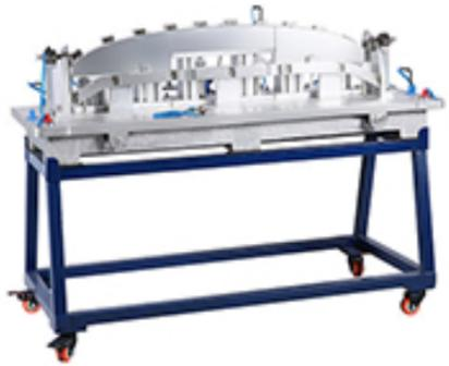
Front bumper lower trim panel checking fixture
